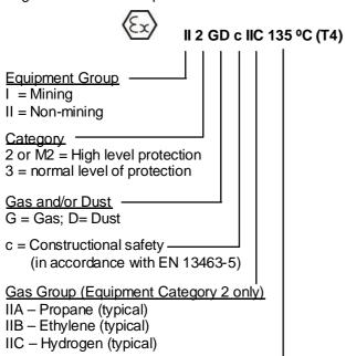
Maximum surface temperature (Temperature Class) (see section 1.6.4.3)
